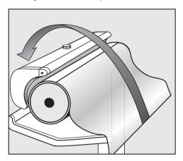
■ Hold the corners of the padding cover, pull taut and keeping taut lay over the heater plate.
